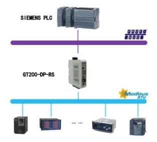
GT200-DP-RS gateway can connect serial devices to PROFIBUS DP fieldbus. GT200-DP-RS gateway is a bridge in the communication network and implements the conversation between serial (Modbus RTU/ASCII and generic) devices and a PROFIBUS DP master.
